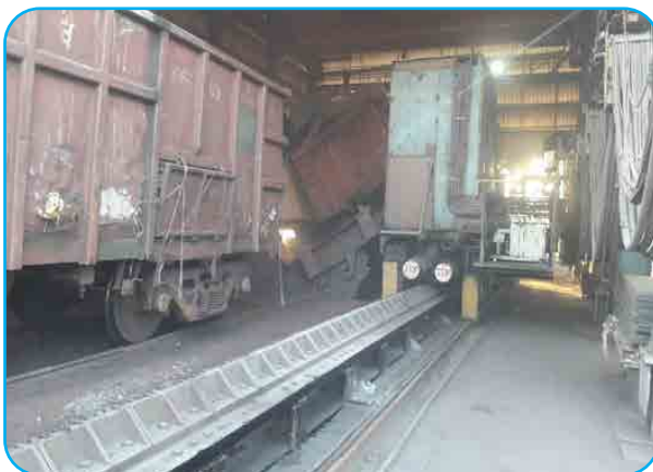
Unloading of wagons at Wagon Tippler
