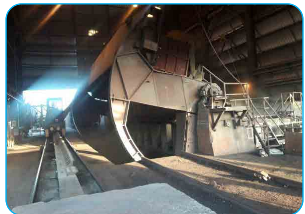
Unloading of wagons at Wagon Tippler
